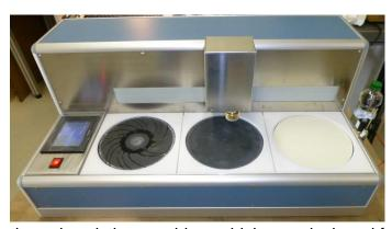
The SPA completes MSC's system for cross-sectioning printed circuit boards. It allows a controlled grinding and polishing to yield specimen ready for optical inspection.
