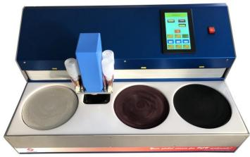
The Multi-Polishing machine MPA can produce high quality polishing results on PCB test coupons. For that job the machine is equipped with 3 polishing plates for running a multi-step polishing process with different polishing cloths together with up to three different polishing liquids. This makes it possible to
