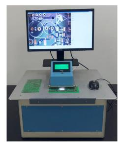
The S-OSR is part of MSC's system (specimen preparation, grinding- and polishing) for microsectioning printed circuit boards (PCB). Our system allows the highly automated preparation of microsections for optical inspection.
